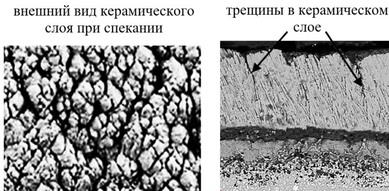
Fig. 2. Appearance of the ceramic layer ZrO_2+8\%Y_2O_3 at the sintering site and when cracks appear
