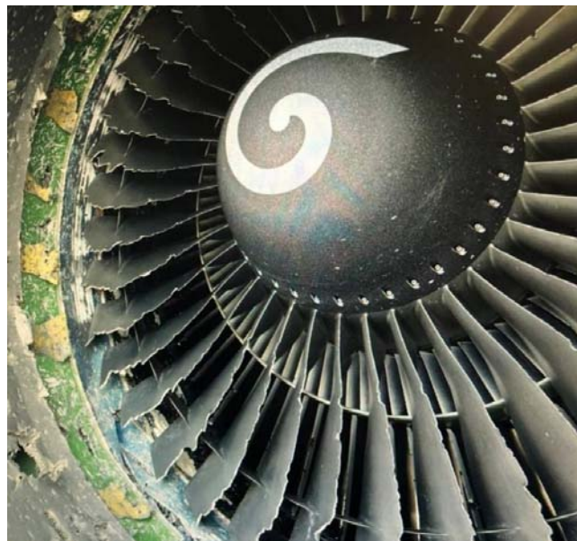
Fig. 2. Destroyed engine as a result of a bird strike
