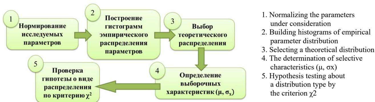
Fig. 3. Methods of the experimental data statistical analysis
