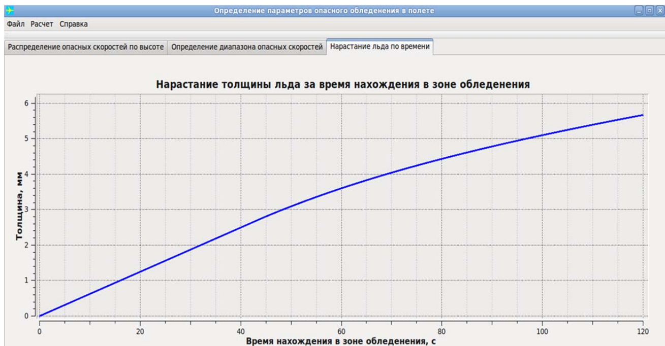
Fig. 4. Dependence of ice thickness on exposure time
