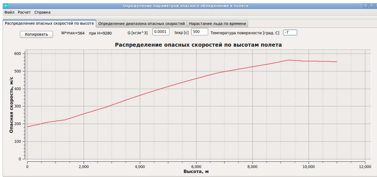
Fig. 2. Flight altitude dangerous velocities distribution
