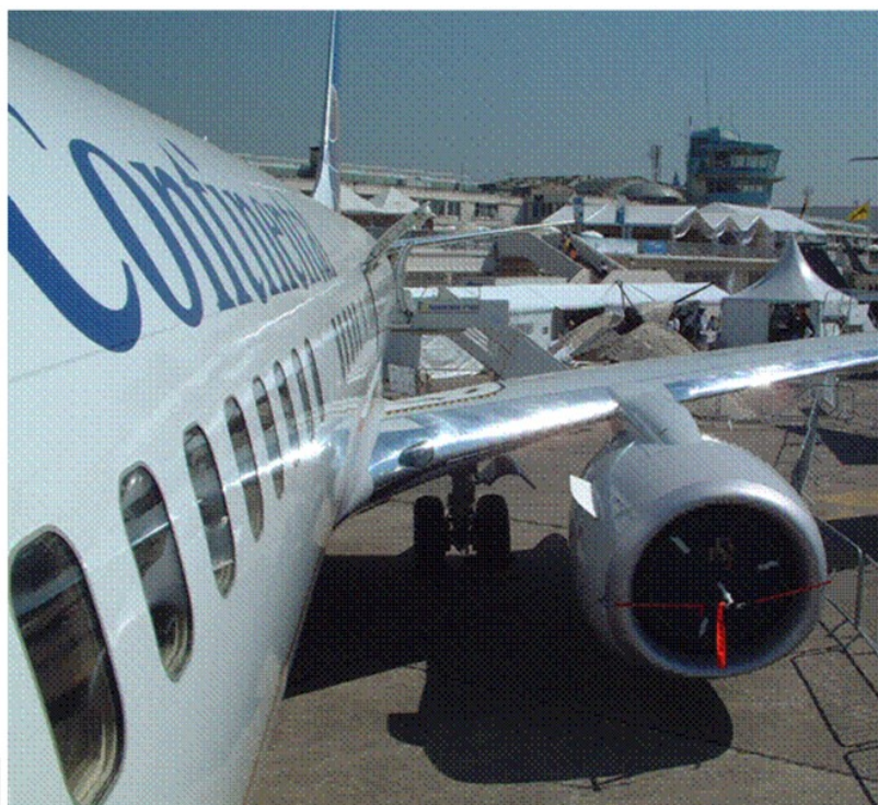
Fig. 2. Vortex generator on the engine nacelle
