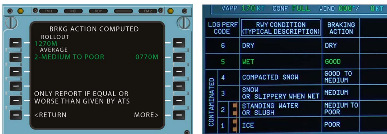
Fig. 4. Example of MCDU screen with the runway status output from BACF
