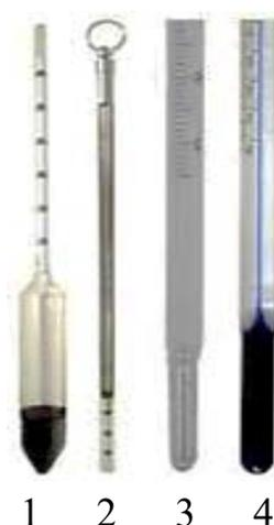
Fig. 5. Aerodrome control devices: thermometers (1, 2) and hydrometers (3, 4)
