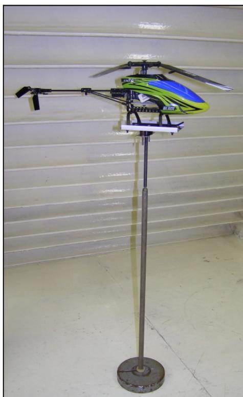
Fig. 1. Helicopter model on vertical strut support
