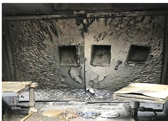
Fig. 4. Appearance of the electron beam installation with ceramic condensation on its walls
