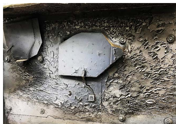
Fig. 4. Appearance of the electron beam installation with ceramic condensation on its walls
