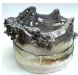
Fig. 2. Appearance of uneven evaporation of the surface of a ceramic rod made of stabilized zirconium dioxide in an electron beam installation
