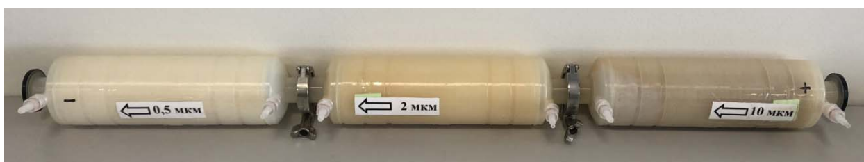
Fig. 5. Water treatment filter
