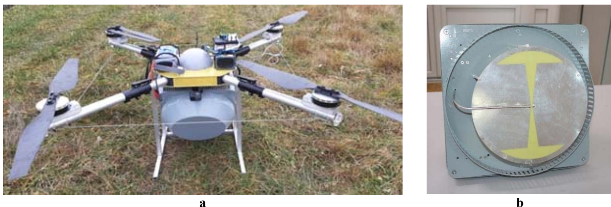
Fig. 7. a – airborne radar reconnaissance complex “Arkheolog”, b – airborne P-band radar “Linza”, dimensions 43×38×27 cm, weight up to 9 kg
