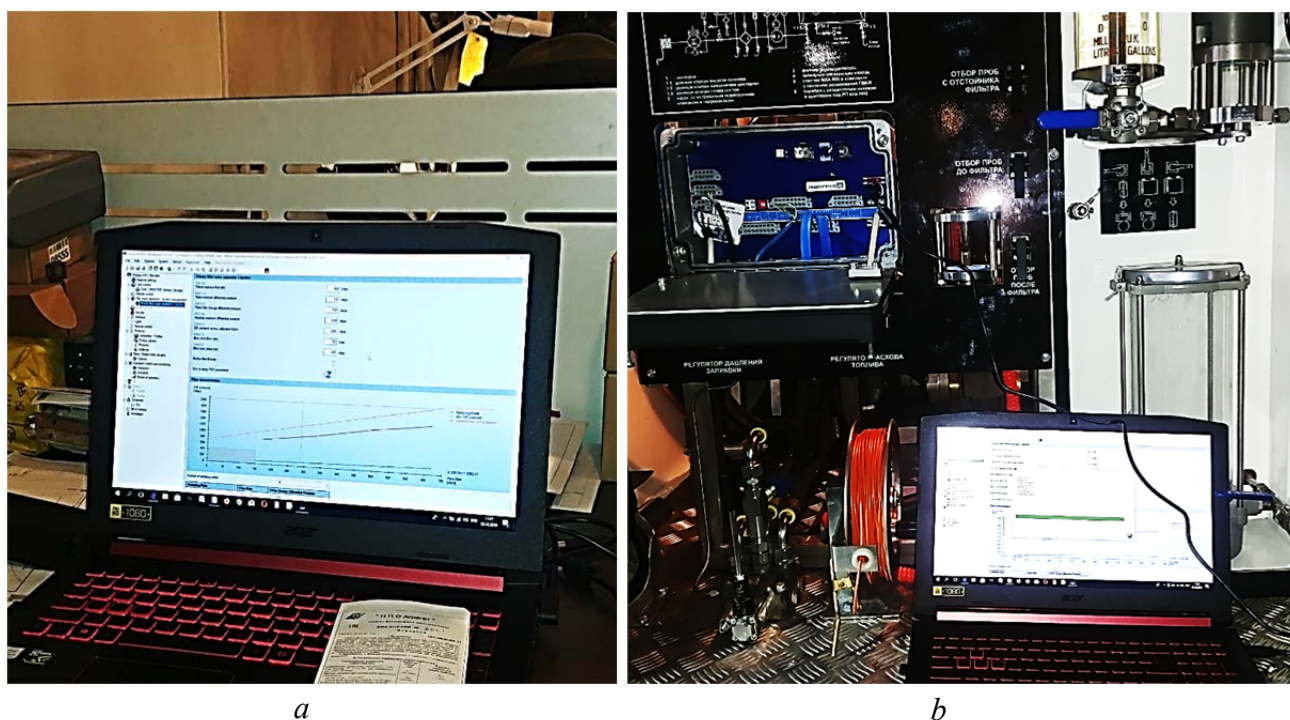
Fig. 6. Differential pressure passport data entry into the computer software (a) and their transmission to the on-board controller software (b)
