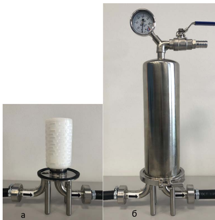
Fig. 2. External view of the filter components a – External view of the replaceable filter elements; б – Filter holder
