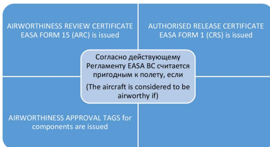
Рис. 8. Условия допуска ВС к полетам по правилам EASA Fig. 8. Conditions for admitting aircraft to operation according to EASA
