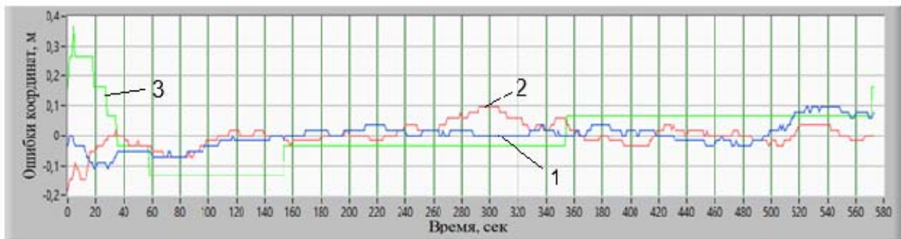
Fig. 10. Positioning errors with interference at the GLONASS frequency
