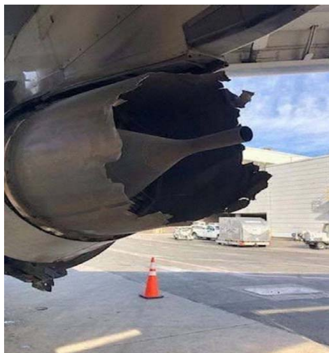
Fig. 3. Destroyed engine nozzle because of a bird strike
