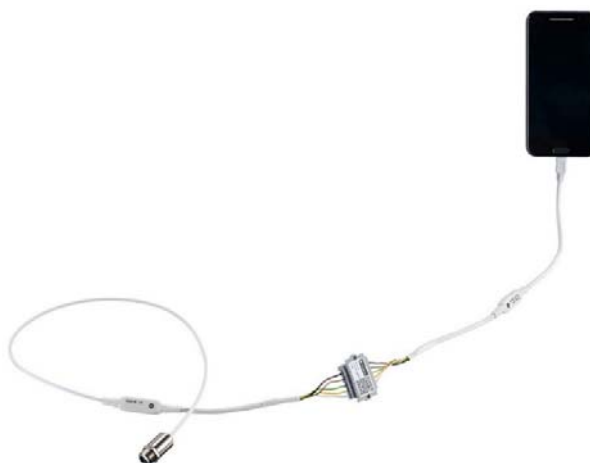
Fig. 2. Pyrometer with a flexible cable and a recording application
