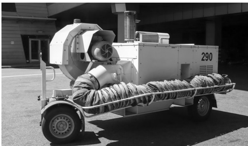
Fig. 1. Hot air source is the engine heater
