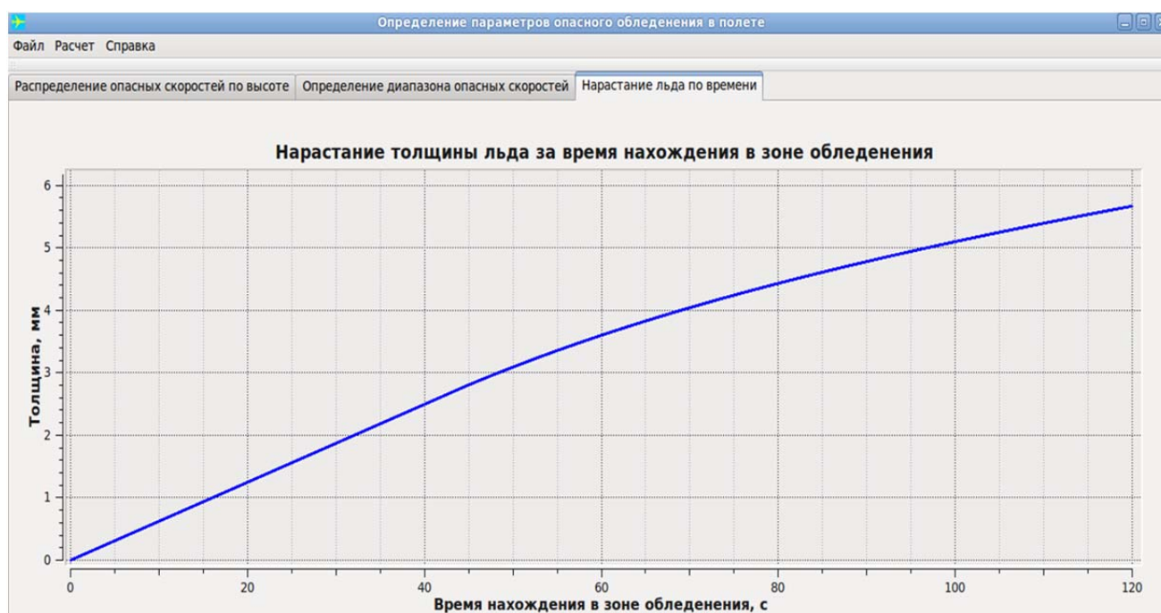
Fig. 4. Dependence of ice thickness on exposure time
