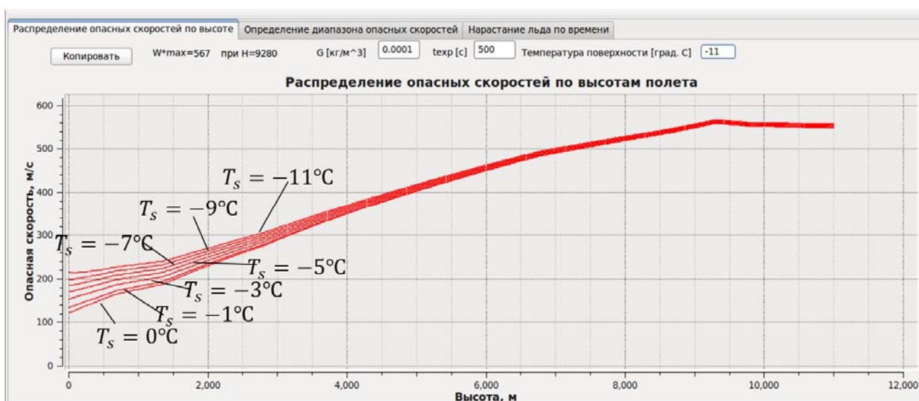
Fig. 7. Surface temperature influence on distribution of dangerous speeds by flight altitude
