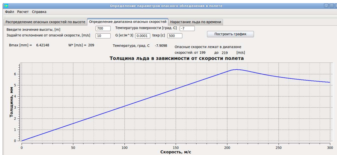
Fig. 3. Determination of the dangerous flight speeds range
