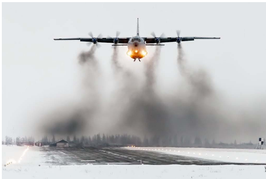
Fig. 1. Random visualization of the wake vortex following the Antonov-12 turboprop aircraft during takeoff
