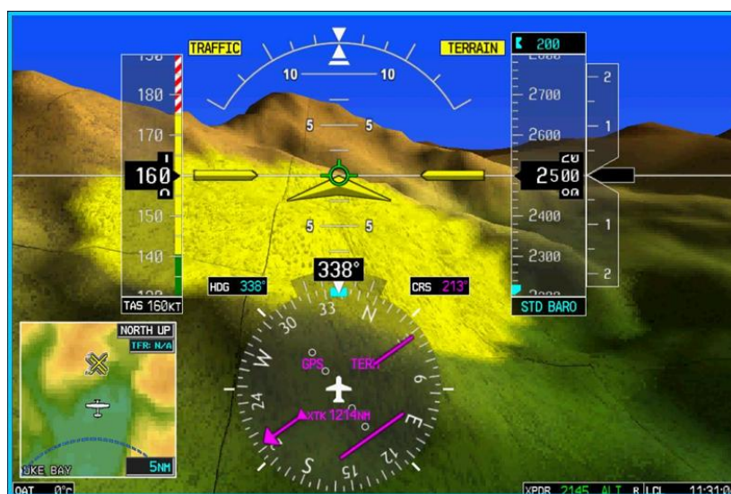
Fig. 8. Example a synthetic vision system display in the Garmin suite
