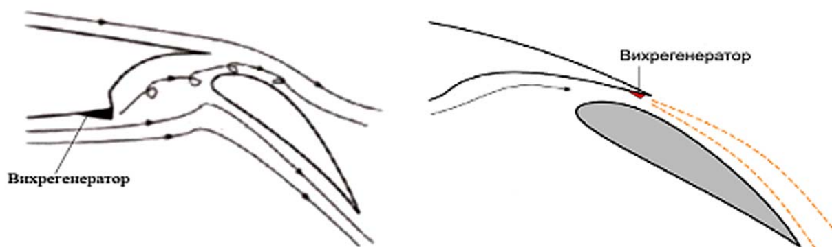
Fig. 4. Various options for installing vortex generators
