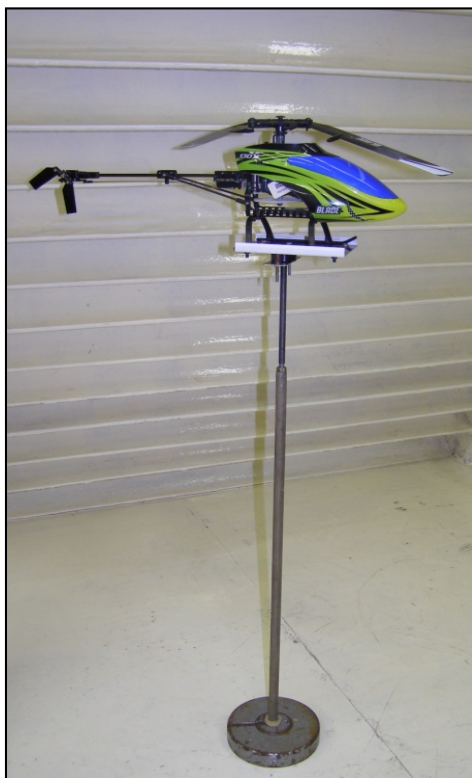
Fig. 1. Helicopter model on vertical strut support
