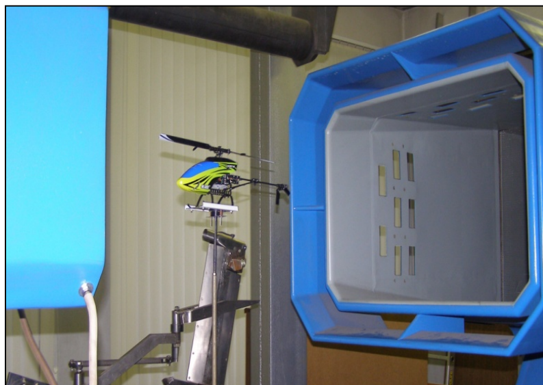
Fig. 2. Helicopter model in the wind tunnel test chamber
