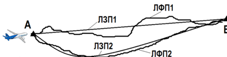
Fig. 1. Desired track for various trajectory holding errors, here Л3П1 – LDP1; Л3П2 – LDP2; ЛФП1 – TMG1; ЛФП2 – TMG2
