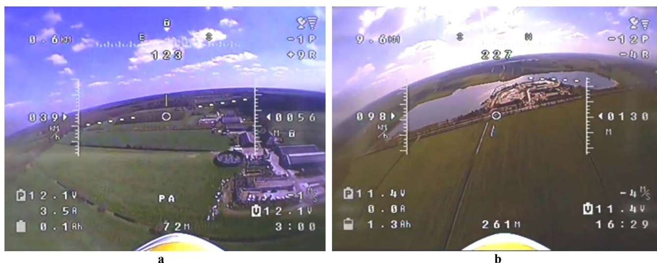
Fig. 6. The results of the registration of images of the terrain by an optical-electronic system when approaching the first landmark (a) and upon approaching the second landmark (b)
